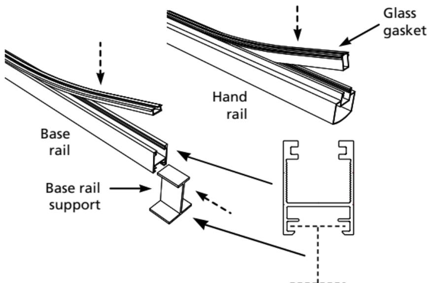
**4** Insert the rails into the posts. Position and fasten the second post in place - ensure that the post is plumb. Secure the rails to the posts with self-drilling screws. (Refer to Step 4 on Page 5.)
