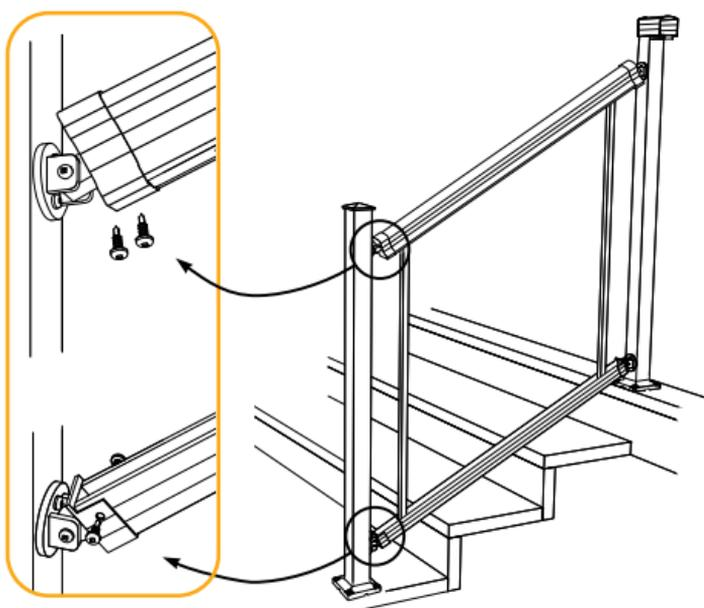
**3** Place a picket into both rails near the bottom post - ensure that the picket is plumb and 4" or less from the post. Starting from the bottom post, measure and cut the **end spacers** then remove the picket (**Fig. 1**).
