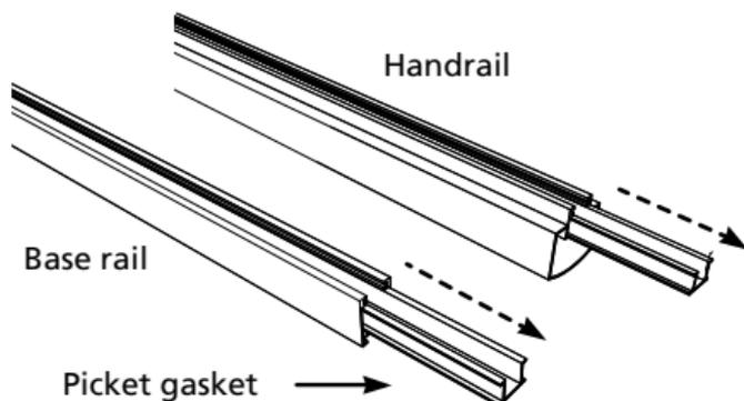
**3** Cut the glass gaskets the same length as the rails and drill 1/8" holes into the base rail glass gasket for water drainage. Press the glass gaskets into the rails and install the base rail support into the bottom channel of the base rail.
